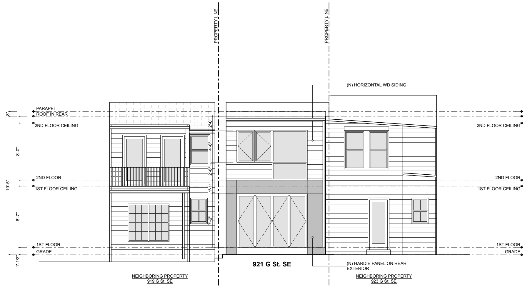
1 A-111 Rear Elevation: Proposed SCALE: 1/4" = 1'-0"
