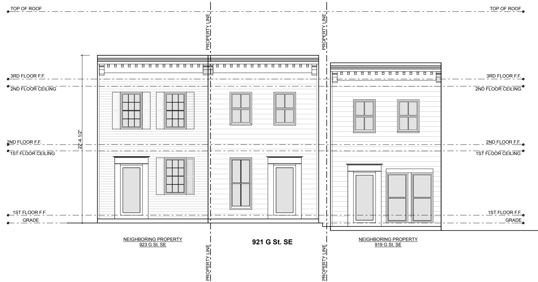
1 Front Elevation: Existing & Proposed A-110 SCALE: 1/4" = 1'-0"
